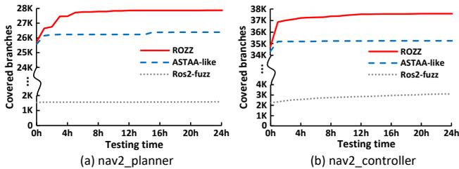
Fig. 7. Growth of covered code branches with the testing time.
